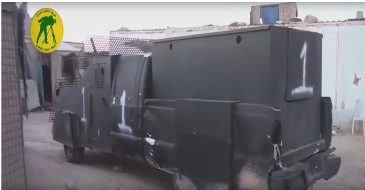
Fig. 1. Car bomb on the basis of a pickup truck. The metal sheets cover the entire body. Protection is provided from RPG hits on the cab through use of a steel grid or mesh.
