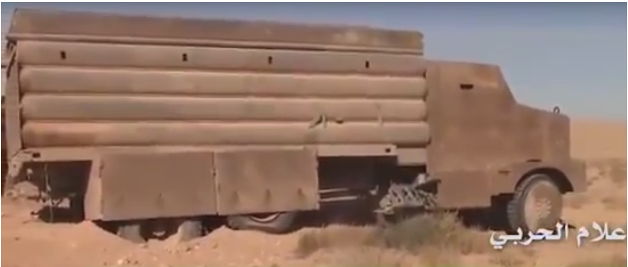
Fig. 4. Car bomb based on a 3-axle army truck. The metal sheets cover the entire body.
