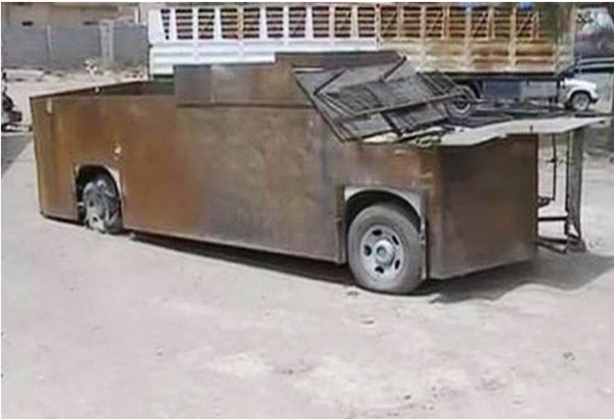
Fig. 2. Car bomb on the basis of a van. The metal sheets cover the entire body.
