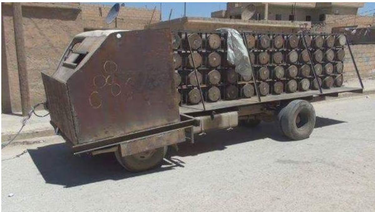
Fig. 3. Shahid-mobility on the basis of a truck. Only the cab is enclosed by armor.
