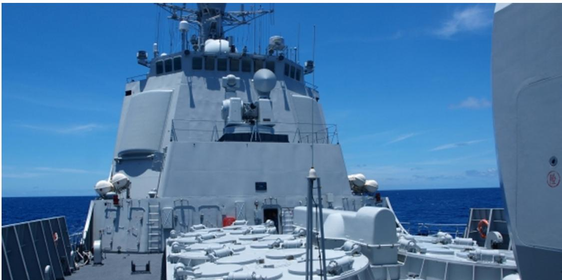
Type 052C picture illustrating convex radar array panels and round VLS 6 cell launchers.
