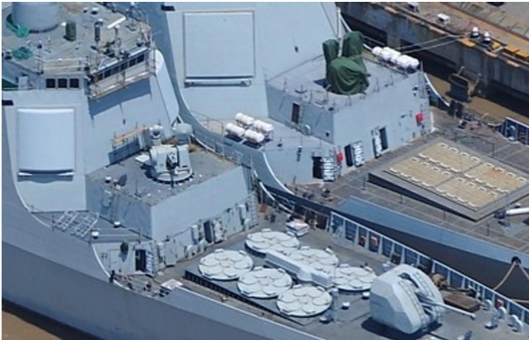
Detail of differing VLS and AESA radar arrays of Type 052C and 052D Class DDGs.
