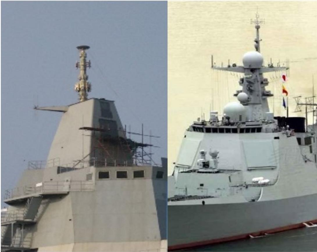
A comparison of the integrated mast structures of the Type 055 mock-up and the active Type 052D Kunming. Note the location of the forward two active phased array radar panels on the Kunming. The large sloped superstructure facing, just under the starboard side bridge deck portals on the Type 55, will be fitted with a similar APAR panel.
