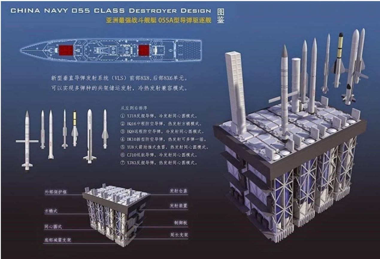
This unofficial artist's rendition illustrates the modular nature of the PLAN VLS and its ability to be loaded with a mix of missiles. This allows the PLAN to equip its vessels with mission specific payloads. The red squares denote the approximate orientation of the two VLS on the Type 055.
